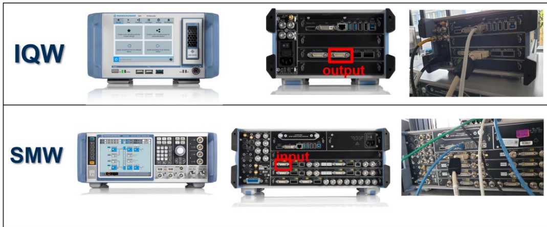
Figure 4.13 Real-world RF Spectrum playback setup
