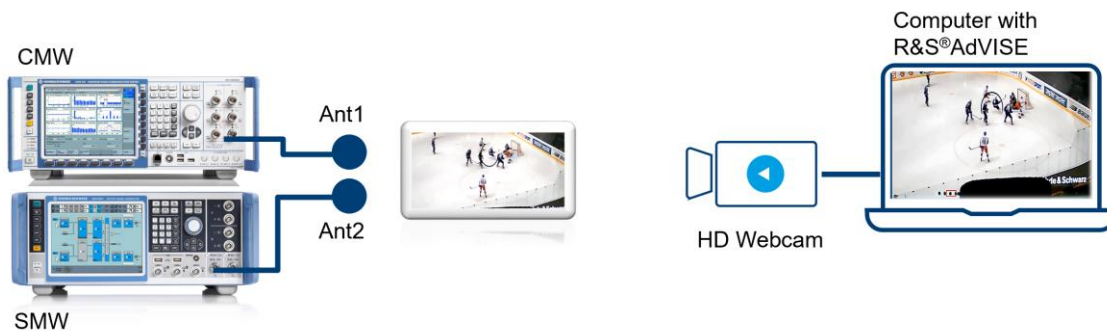
Figure 4.14: Measurement Setup for detecting video disturbances caused by RF interference signal
