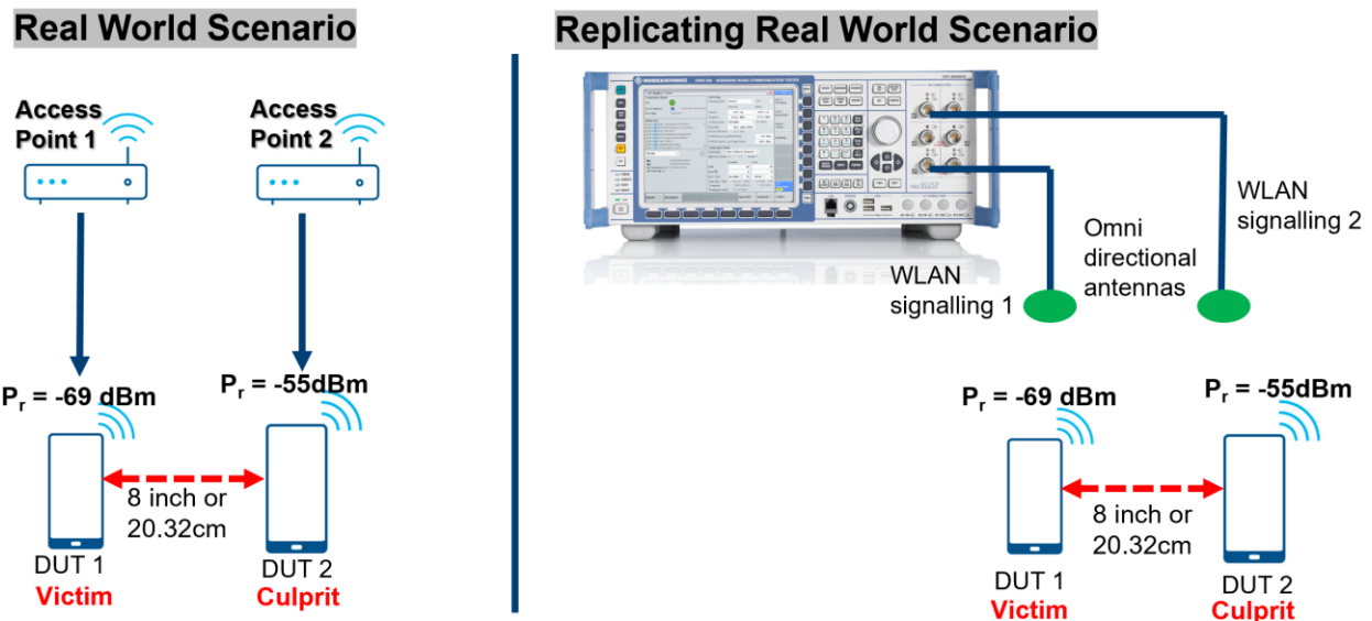
Figure 4.5: Real world scenario mutual interference effect recreated in the test chamber
